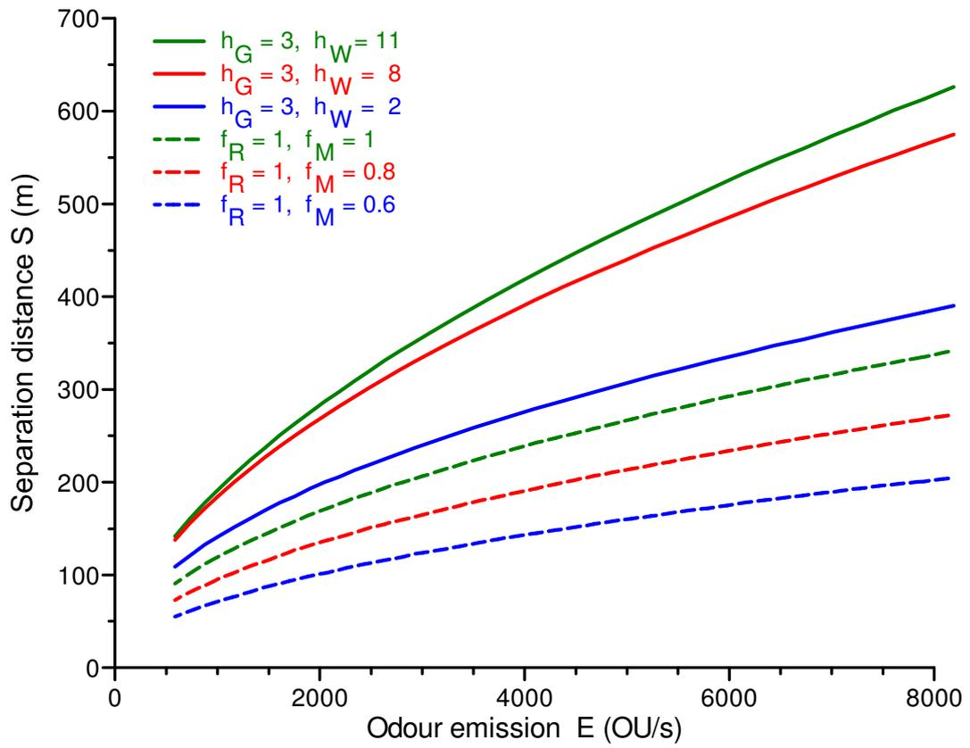
**Figure 1.** Comparison of the separation distances for pure residential areas (empirical model:  $h_G=3\%$ , solid lines, guide line:  $f_R=1$ , dashed lines)
