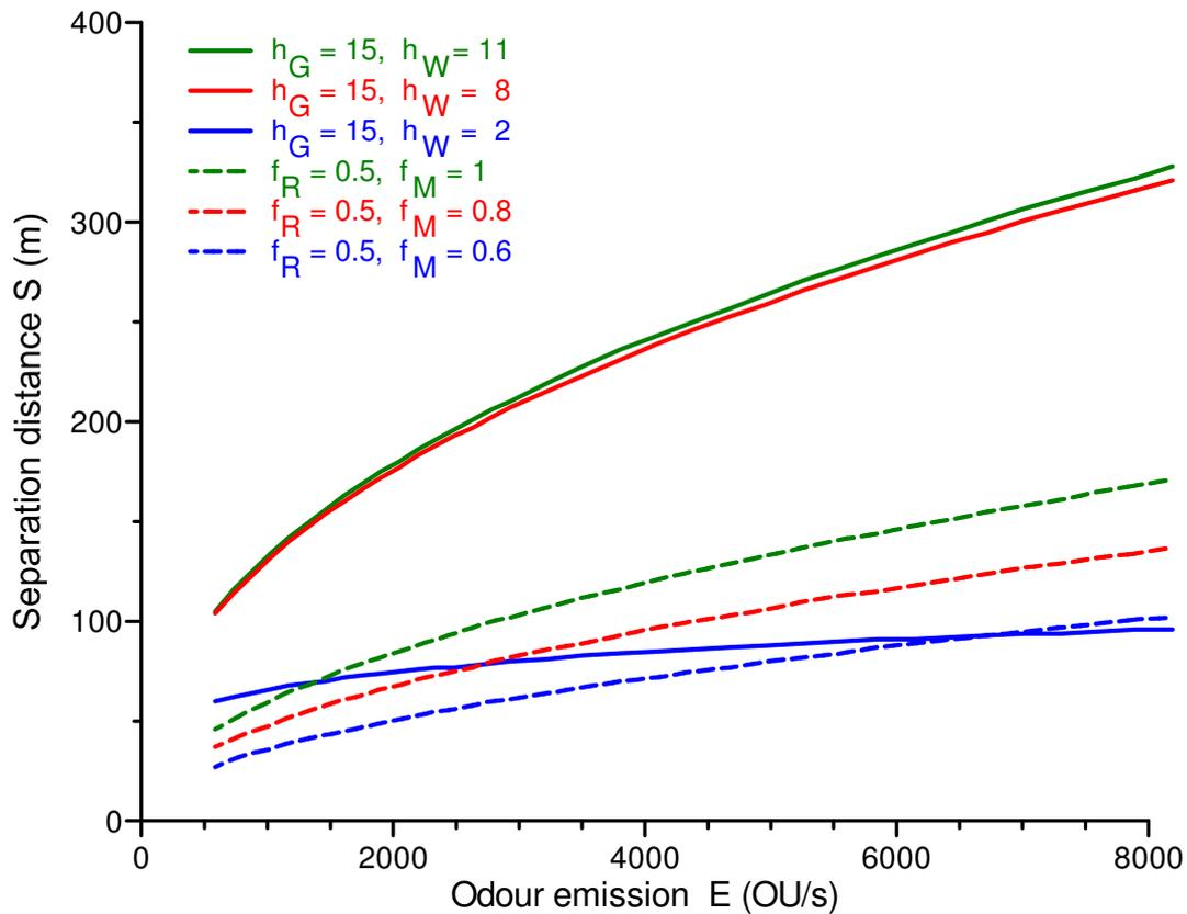
**Figure 3.** Comparison of the separation distances for areas of mixed residential/commercial activity (empirical model:  $h_G=15\%$ , solid lines; guide line:  $f_R=0.5$ , dashed lines)
