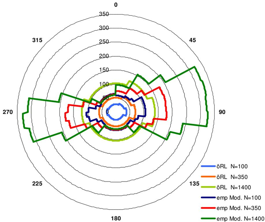
**Figure 6.** Comparison of separation distances for areas of mixed residential/commercial activity ( $f_R = 0.5$ ) between the Austrian guide line (öRL) and the empirical model ( $h_G = 15\%$ ) for three livestock units ( $N$  = number of fattening pigs)
