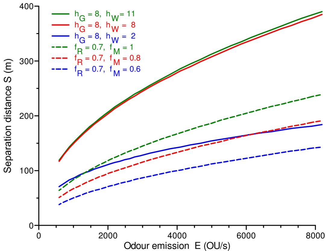
**Figure 2.** Comparison of the separation distances for common residential areas (empirical model:  $h_G=8\%$ , solid lines; guideline:  $f_R=0.7$ , dashed lines)
