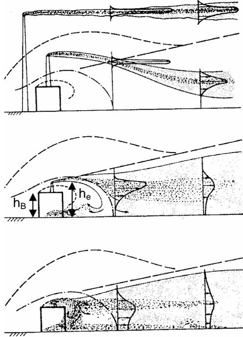
Fig. 4: Influence of the height of the odour emission  $h_e$  compared to the building height  $h_B$  [after [8]]
