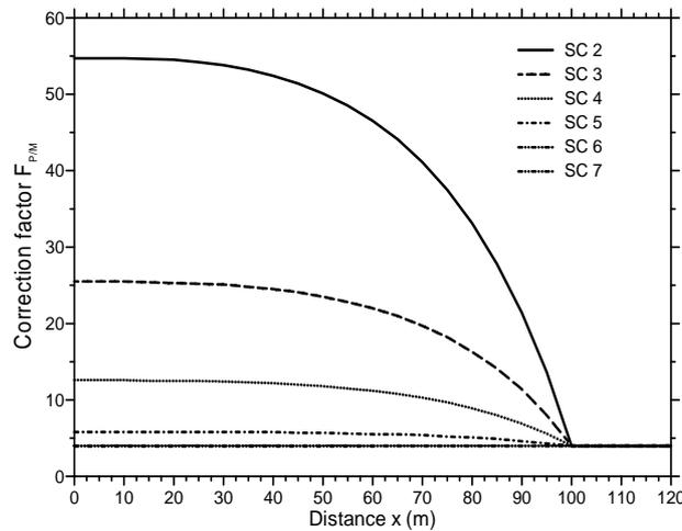
Fig. 1: Correction factor  $F_{P/M}$  as a function of the distance from the source  $x$  (m). The graph shows a maximum for stability class  $SC = 2$  and a value  $F_{P/M,max} = 4$  according to ODIF or AUSTAL 2000G.
