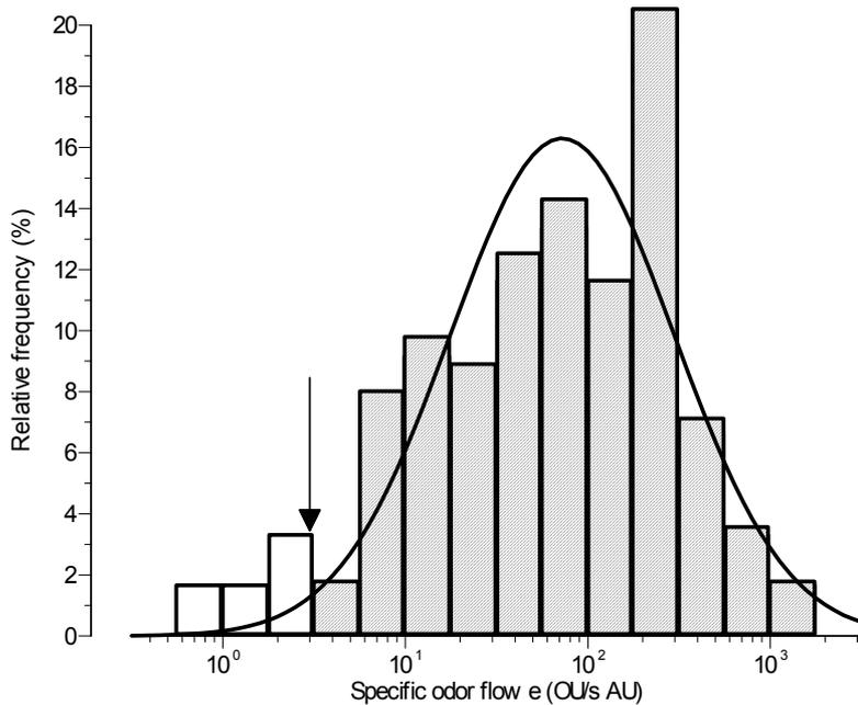
**Fig. 1: Relative frequency distribution of the measured specific odour emission  $e$  in OU/s-AU of the four buildings and a log-normal distribution with a mean of 1.86 and a standard deviation of 0.61. The arrow marks the cut-off values of outliers, which were eliminated for subsequent data analyses (empty bars)**
