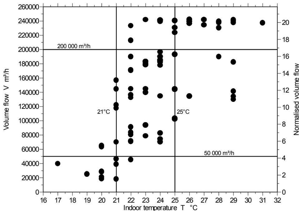
**Fig. 2: Scatter diagram of ventilation airflow and indoor temperature. The lines show the limits for dividing the overall data set into three subsets to eliminate influence of confounders. On the right y axes, the ventilation rate  $V_n$  is normalized by product of the number of animals ( $N_d=1000$ ) with the minimum ventilation rate per animal for winter time ( $V_d=3.31 \cdot 10^{-3} \text{ m}^3/\text{s}$ )**
