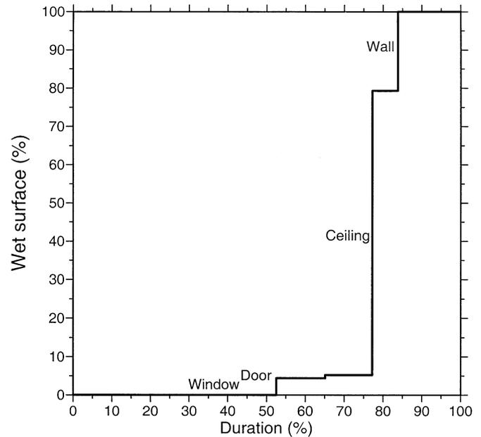
**Fig. 4** Portion of wet surfaces of the inside areas of the livestock building as a function of the duration (%) of condensation. The wetted surface areas of the building elements are summarised in Table 3
