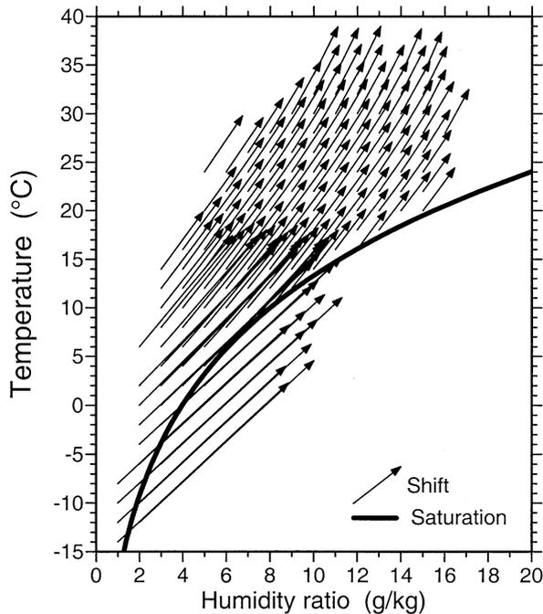
**Fig. 3** Psychrometric chart of the indoor and outdoor air conditions. The vectors show the change of air temperature and humidity ratio due to the livestock, the building and the ventilation system. Tail of the vector: outside situation, head: indoor. For the heads of the vectors below the saturation curve a relative humidity of 100% and condensation of the surplus of humidity is assumed
